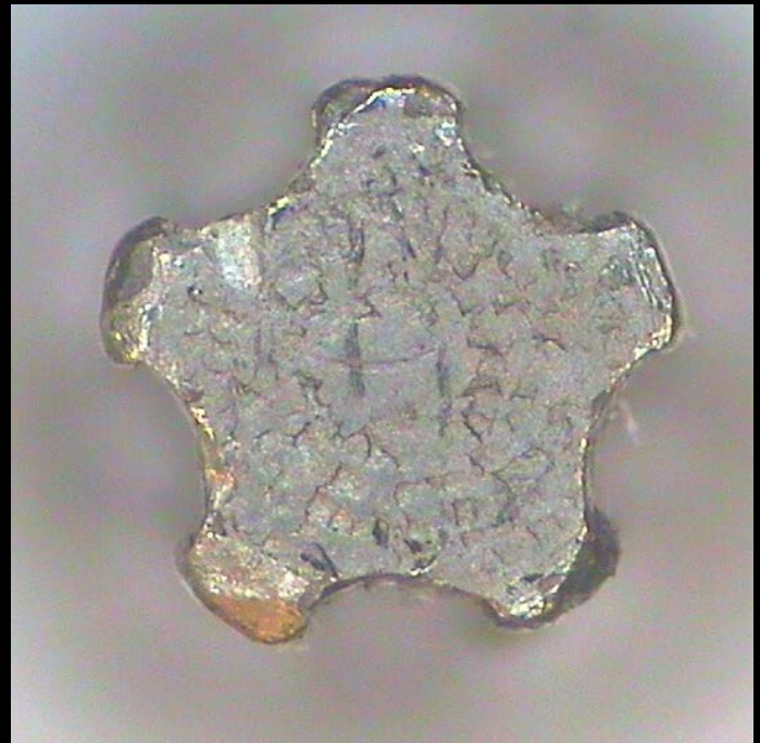
Standard drive bit production: underfilled and severe edge rounding minimises fit and performance.
