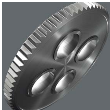
Zyklop Metal Switch Fine-tooth mechanism with 72 teeth for a return angle of only 5°. This short stroke allows fast and precise work in all types of installation.
