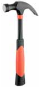
891 Claw Hammer American Pattern, face diameter 25 or 27 mm, 16 or 20 oz.
