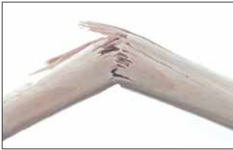
As a result of its long fibres, the hickory wood used on the shaft of the SecuTec® hammer keeps the shaft together in the event of it breaking.
