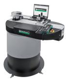
Fully-automated calibration and adjustment of torque and angle using the perfectControl calibrating unit No 7794-3.
