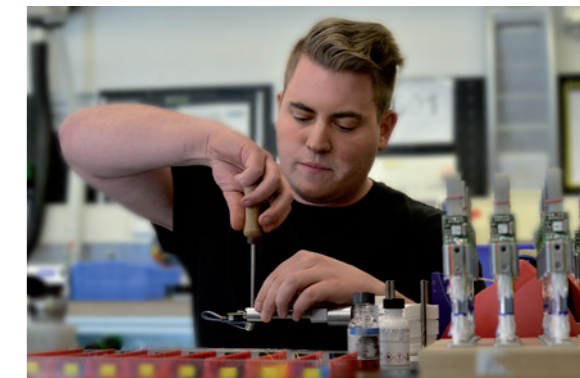
Torque wrenches by STAHLWILLE – assembled by hand to meet and exceed the highest standards.
